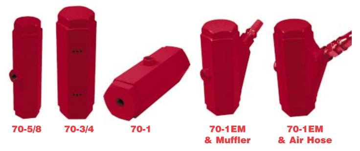
Model 70 end-mounted series pneumatic piston vibrators produce a linear force with frequency and force adjustable with air pressure. A self-starting spring is installed for fast start in any position. A variety of options are available. The mounting hole can be supplied with an M-millimeter thread or US standard NF (National Fine) thread.
